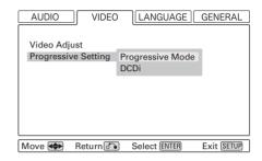
The progressive-scan mode setting menu has two sub-menus: Progressive Mode (progressive scan mode) and DCDi.
